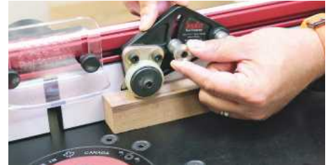
▲ These 'Clear Cut' Stock Guides are superb and incorporate anti-kickback wheels
